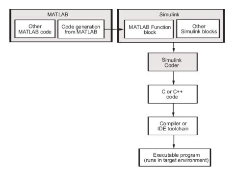
The code generation workflow is a part of the V-model on page 1-6 for system development. The process includes code generation, code verification, and testing of the executable program in real-time. For rapid prototyping of a real-time application, typical tasks are:
